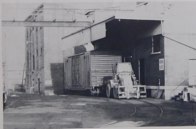
When a switcher is not available, Carbon Sales moves boxcars using a front-end loader which sports a coupler. Here, the front-end loader is about to move a boxcar filled with packaged culm coal away from the storage and loading building so that it can be handled later in the day by a PNER locomotive.
