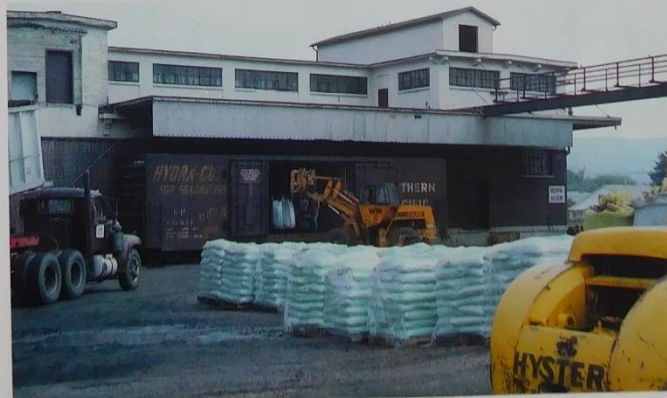
A busy day at Carbon Sales. With numerous 100-lb. sacks waiting nearby, a front-end loader transfers a one-ton bag to a double-door boxcar. Inside the car a forklift positions the loads for transit. At left, a truck dumps a load of processed culm coal from the Culmtech plant into a bulk storage pile.
